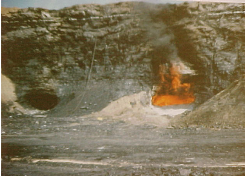
Figure 12: Open bords in which spontaneous combustion has occurred
