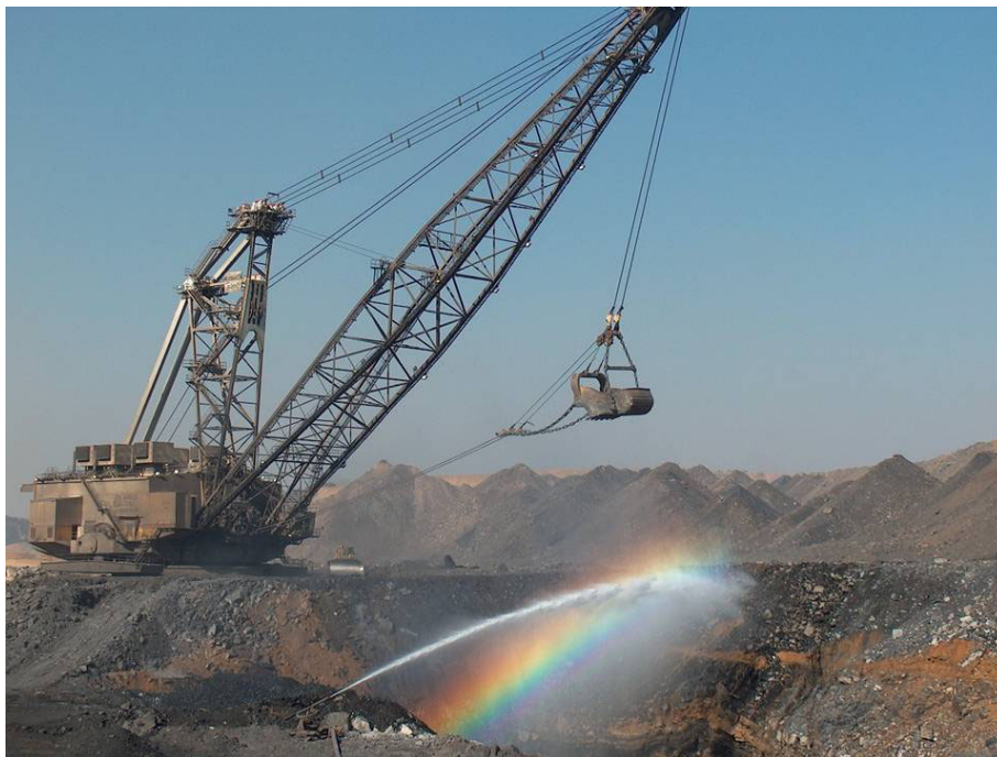
Figure 20: Reducing dust and haze caused by hot material
