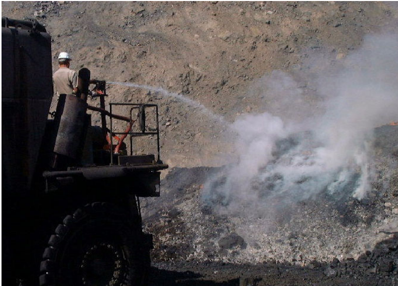
Figure 19: Spraying of hot coal using a water cannon before loading coal into the trucks
