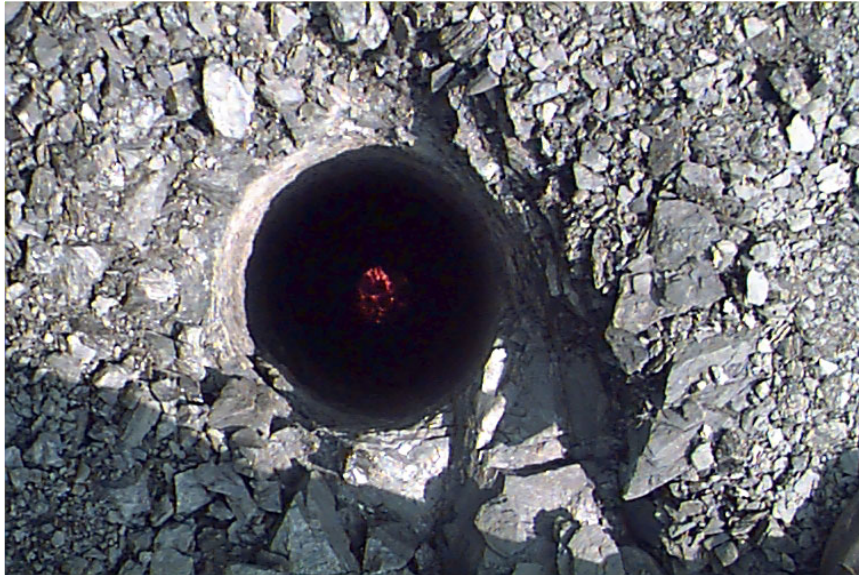
Figure 18: View down a hot hole
